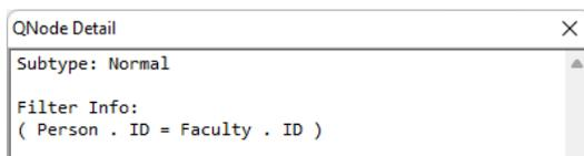
This filter ensures that **ONLY** those combinations of records where **Person.ID** is equal to **Faculty.ID** will pass up to the Join above it, effectively creating an **INNER JOIN**, also known as an **EQUAL JOIN**.
